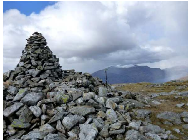
Survey point next to the cairn on Leum Uilleim, showing the top of the cairn to be about 2m above the top of the pole
